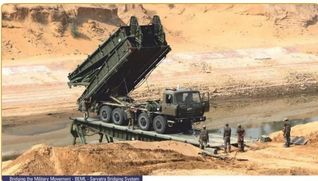
Sarvatra: truck-mounted multi-span mobile bridge in action.
